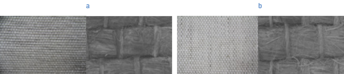
Figure 5. Flax fabrics with the plain weave, made from the 68 tex low-twist yarn (warp) and from natural (a) and bleached (b) rovings of the linear mass of 2000 tex (weft), and microscopic images of fabrics – under the scanning electronic microscope with changing vacuum mode.
