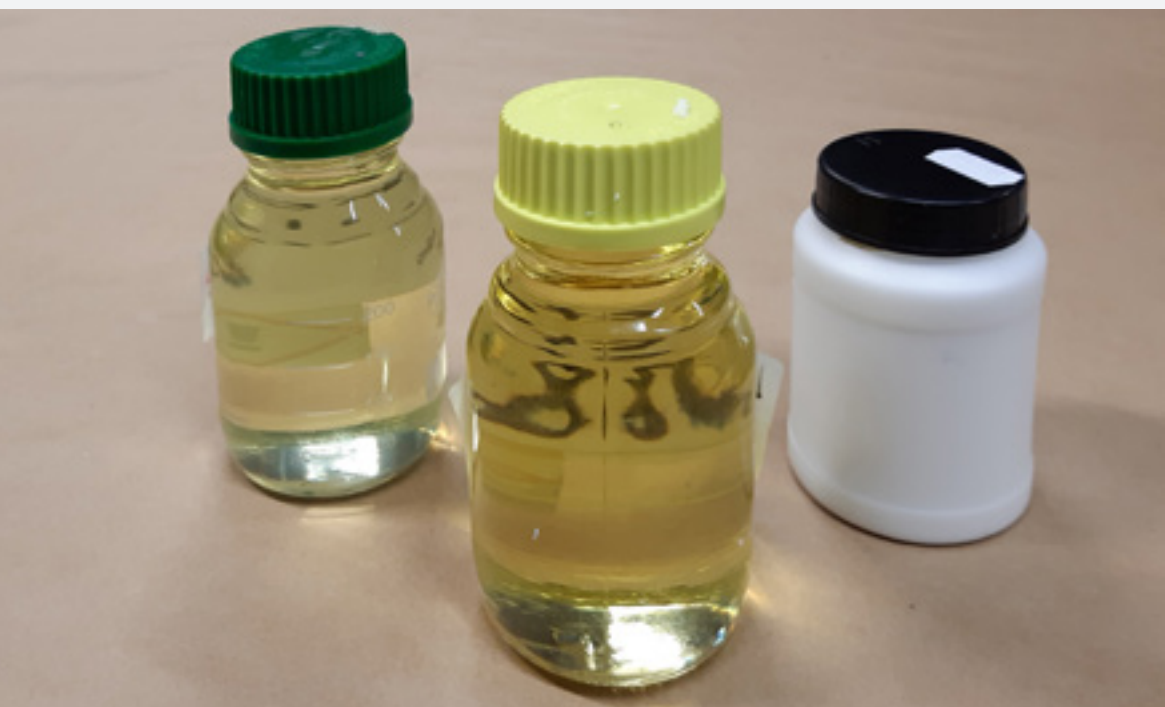
Figure 9. Epoxy resin based on linseed. It consists of: modified epoxy, hardener, flame retardant.
