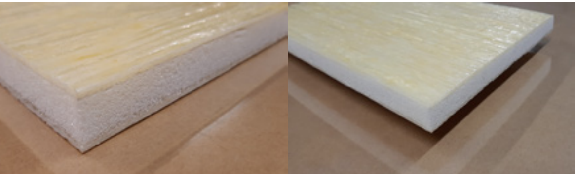
Figure 10. Sandwich construction with decking layer made out of natural fibre composite from bleached flax-fibre and linseed based epoxy
